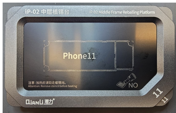
Picture Ref 6.2.21: RF Logic Board Reball – Stencil.JPG
